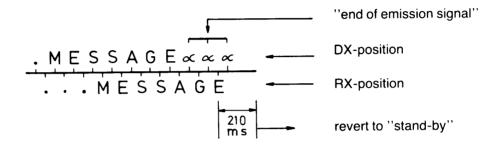
3.2.7.3 The CBRS or the SBRS reverts to the ''stand-by'' position not less than 210 ms after receipt of at least two consecutive ''idle signals a'' in the DX position.
